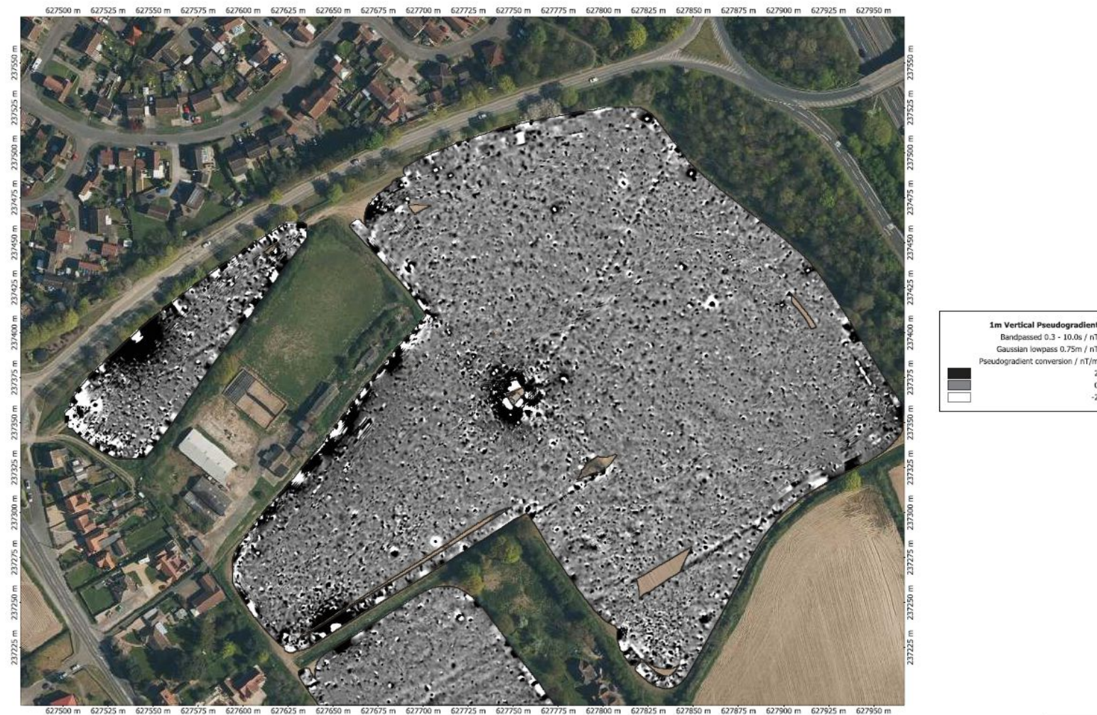
TSM171 Land off Howlett Lane, Trimley St Martin, Suffolk DWG 03a Magnetic Data - 1m Vertical Pseudogradient - North
